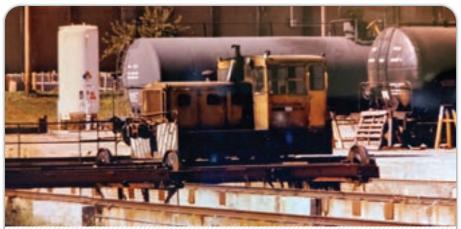
A gas-electric industrial switcher takes a ride on the transfer table at the Cargill plant in Atchison, Kan., in this 1990s-era photo. Mark Huff photo
