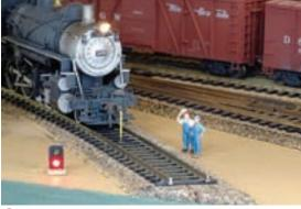
Obve added a red light-emitting diode (LED), mounted in a dwarf signal housing, to the circuit to provide a more visible indication that the bridge was out and the blocking wire was raised.
