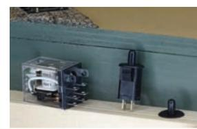
2 Dave used Forstner bits to countersink the normally open plunger switch into the lift bridge's stop block. When the bridge is down, the switch is closed, changing the polarity of the power to the Tortoise and retracting the wire.
